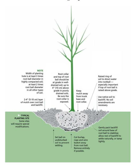
One of the primary causes of tree failure is improper planting depth. Make sure that the root flare is at grade, so that the roots are underground and the trunk is above ground.
